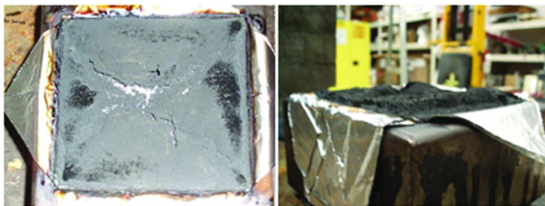
Figure 8. Post Desmopan-5% CNF cone calorimeter sample. Reprinted with permission from ref. (4). Copyright 2011 American Institute of Aeronautics and Astronautics.
