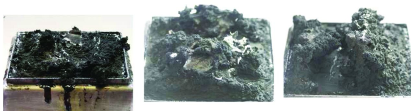
Figure 7. Cone calorimeter residues for PC/ABS + BDP (left), PC/ABS + 10 wt.% talc (middle) and PC/ABS + BDP + 10 wt.% talc (right) at a heat flux of 35 kWm -2 .
