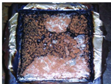
Figure 9. Post Desmopan-5% MWNT cone calorimeter sample. Reprinted with permission from ref. (4). Copyright 2011 American Institute of Aeronautics and Astronautics.
